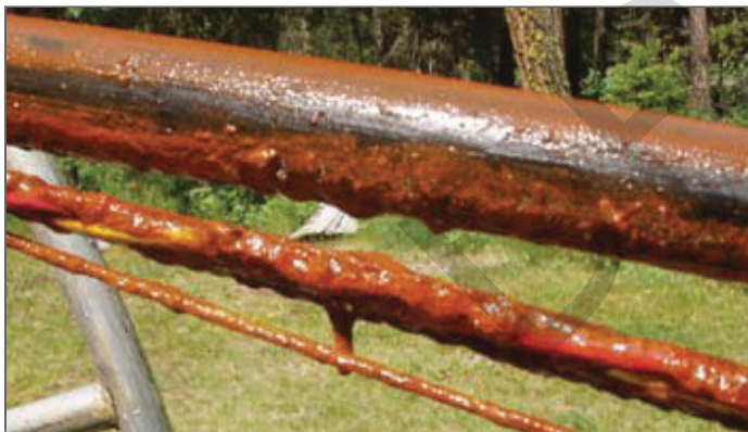
FIGURE 3 Biofilm on well wiring
