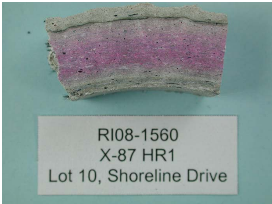
Figure 14: View of Sub-sample X-87 HR1 shown in Figure 12 after polishing and phenolphthalein indicator "staining" (hydrostatic fracture shown at left). The pink colouration indicates a band of unleached (sound) pipe wall.
