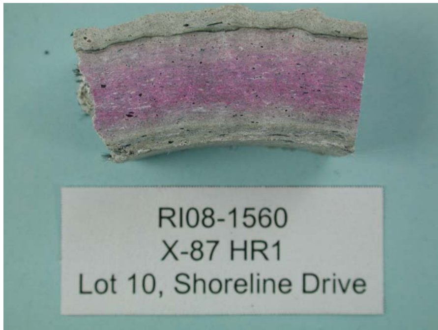
Figure 15: View of Sub-sample X-87 R1 shown in Figure 13 after polishing, phenolphthalein indicator “staining”, drying and marking for SED/EDS analysis.
